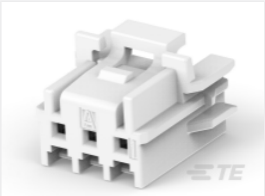
TE 产品编号1-2350224-3 SGI 2.0 Plug Housing, 3 Position, Key A
