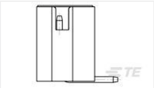
TE 产品编号1775317-7 HPL.,2.5MM PITCH,V/T,SMT TYPE,7 POS
