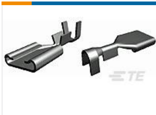
TE 产品编号61202-1 250 FASTON REC 26-22 AWG BR
