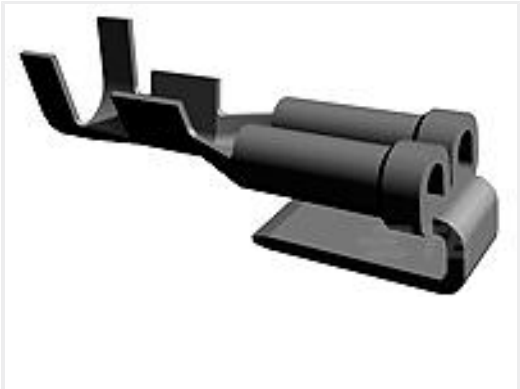
TE 产品编号62003-1 110 FASTON REC 22-16 AWG BR
