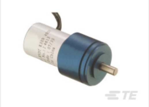
TE 产品编号02560234-060 RVDT R30D +/-60 DEGREE
