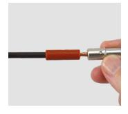
**Step 3:** Insert wire into barrel of contact and crimp using designated tooling.
