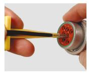
**Step 3:**Pull contact wire assembly out of connector.
