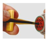
**Step 1:** With rear insert toward you, snap appropriate size removal tool over the wire of contact to be removed.
