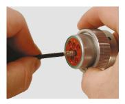
Step 2: Hold connector with the rear grommet facing you.
