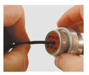
Step 3: Push contact straight into connector grommet until a positive stop is felt. A slight tug will confirm that it is properly locked in place.
