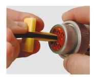
Step 2: Slide tool along the wire into the insert cavity until it engages contact and resistance is felt.
