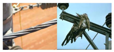
Figure 1. Damage to conductor known as "stranding". Figure 2. Dead bird fallen away from contact area.
