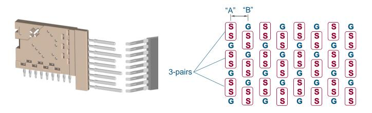
Figure 6. The Fortis Zd design benchmarked the Z-PACK TinMan connector, which is capable of data rates of 12+ Gb/s. Each differential pair in a column is separated by a ground contact.
