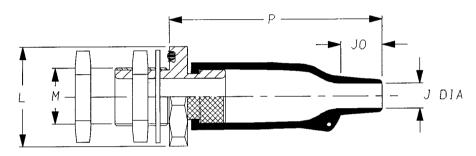
KITS TO INCLUDE CLEANING TISSUE, 1 PIECE 100 GRIT EMERY CLOTH & S1125 ADHESIVE KIT 5. KIT TO BE USED IN CONJUNCTION WITH TCFS INSTALLATION PROCEDURE.
