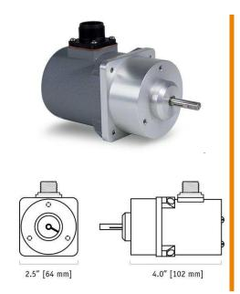
Our model RT8DN communicates rotational position feedback via DeviceNET® to your programmable controller. The heart of this sensor is a precision plastic-hybrid position potentiometer which provides an "absolute" position and does not ever have to be reset to a "home" position after a power loss or planned shutdown.
