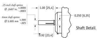
DIMENSIONS ARE IN INCHES [MM] tolerances are  $\pm 0.02$  in. [ $\pm 0.5$  mm] unless otherwise noted
