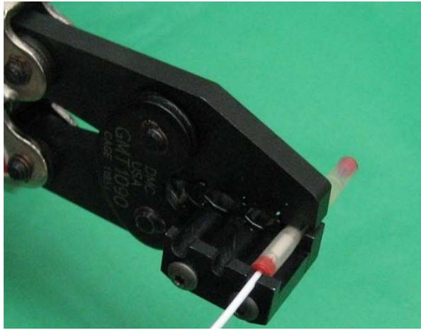
**Picture 3.** Splice location on Tyco Electronics AD-1381 crimp tool
