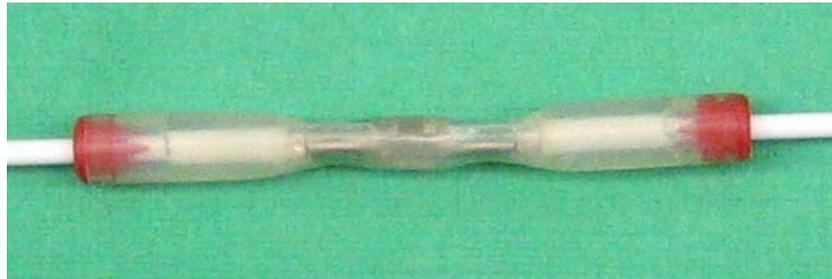
**Picture 6. Crimped conductor**
