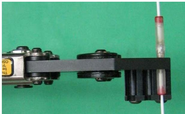
**Picture 4.** Splice location on Tyco Electronics AD-1381 crimp tool, opposite end.
