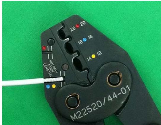
**Picture 1.** Conductor jacket stripped length verification
