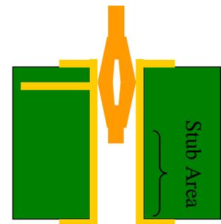
**Figure 7: Via Stub**
