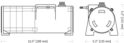
The PT9301 is a combination position and velocity transducer for demanding long-range applications requiring a linear position measurements in ranges up to 1700". A precision plastic-hybrid potentiometer provides accurate position feedback while a self-generating DC tachometer provides a velocity signal that is proportional to the speed of the traveling stainless-steel measuring cable.
