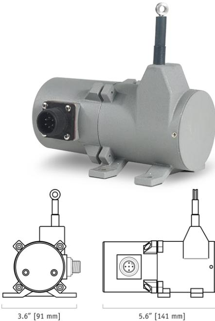
The PT8CN, using a high cycle plastic-hybrid potentiometer, communicates to your PLC via the CANbus SAE J1939 interface. Suitable for factory and harsh environment applications requiring linear position feedback in ranges up to 60".
