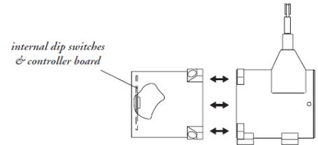
to gain access to the controller board, remove four Allen-Head Screws and remove rear cover.
