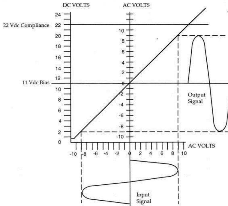
In reference to the illustration above, the compliance voltage is available at 22 Vdc. The bias voltage is set by the accelerometer internal preamplifier at 11 Vdc, and the sensor produces an 18V pk-pk input signal. Under these conditions, the internal preamplifier can produce a distortion-free 18V pk-pk output. However, distortion (otherwise known as clipping) may occur with one or more of the following conditions:
