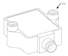
Mounting screws and washers Torque to 3 lb-in (0.3 Nm)
