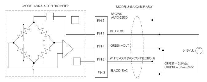
Model 340A cable can also be used if auto-zero function is not required.
