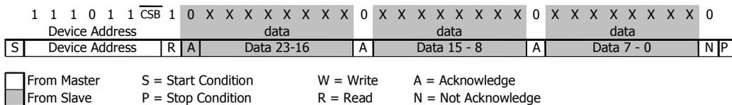
Figure 12: I<sup>2</sup>C pressure response (D1) on 24 bit from MS5803-01BA07
