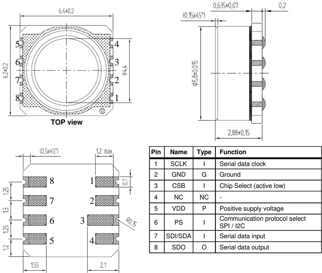
Figure 17: MS5803-01BA07 package outlines, pin configuration and description
