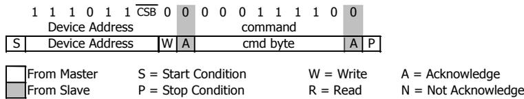
Figure 9: I<sup>2</sup>C Reset Command
