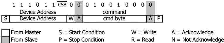
Figure 10: I<sup>2</sup>C Command to initiate a pressure conversion (OSR=4096, typ=D1)
