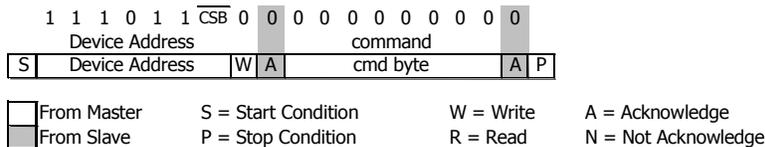
Figure 11: I<sup>2</sup>C ADC read sequence
