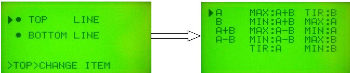
Use the [▼] [▲] [▶] buttons to select the parameter to be displayed, and then press [MENU] or [ENTER] to exit. In RUN mode, the display will automatically show two items. If an actual value is larger than the full scale value (over-range), the warning "FS" will display above the appropriate item:
