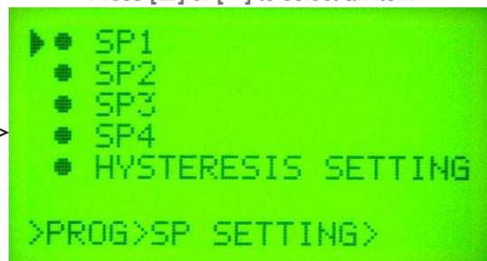
The following are the submenus for the Set-Point Settings (same submenus for SP1, SP2, SP3, & SP4):
