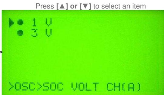
*Note: The oscillator voltage setup menu is the same for CH(B). Each channel can be setup for a different oscillator voltage or the same. However, the oscillator frequency is common for both channels.*
