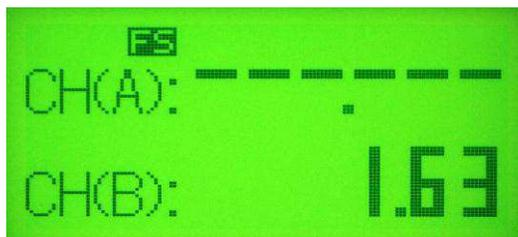
In the RUN mode, pressing [ENTER] will enable the one item display mode. Pressing [ENTER] again will toggle between CH(A) and CH(B). Single channel display mode with CH(A) selected is shown below:
