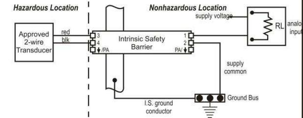
Figure 2. Return Lead Grounded
