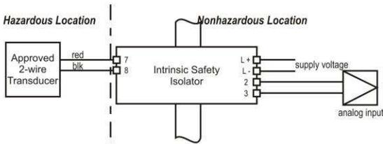
Figure 3. Field Circuit Isolated
