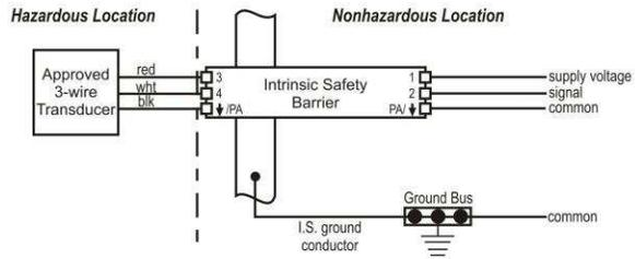
Figure 4. Wiring diagram for 3-wire, VDC output.
