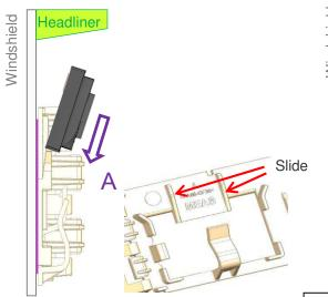
Priming insertion: apply against the slides to control the displacement following "A".
