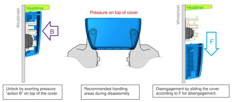
System is designed to support 5 Assembly/Disassembly of cover.
