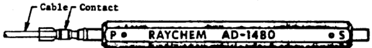
AD-1480 Repair Holding Fixture With Contact / Cable Assembly (Outer Pin Contact Shown For Reference)
