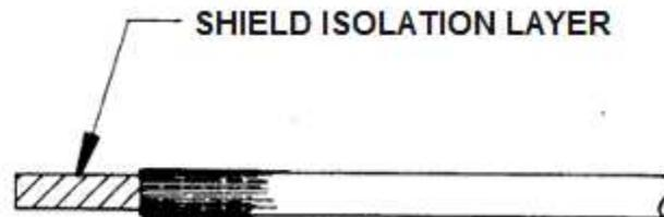
5. Remove any inner jacket and/or shield isolation layer back to the folded braid.
