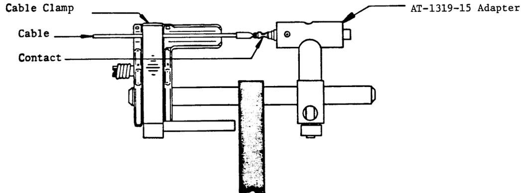
**Figure 5****AD-1319 Holding Fixture and AT-1319-15 Adapter with Contact/Cable Assembly**
