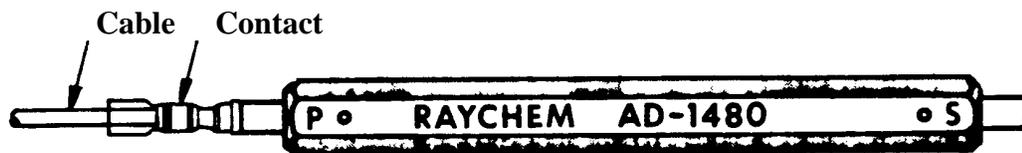
**AD-1480 Repair Holding Fixture with -Contact/Cable Assembly
