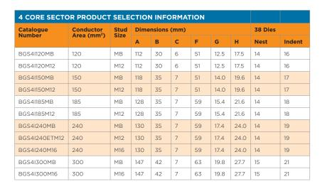
ET - Electro tinned finish Note stud size "MB" means blank palm
