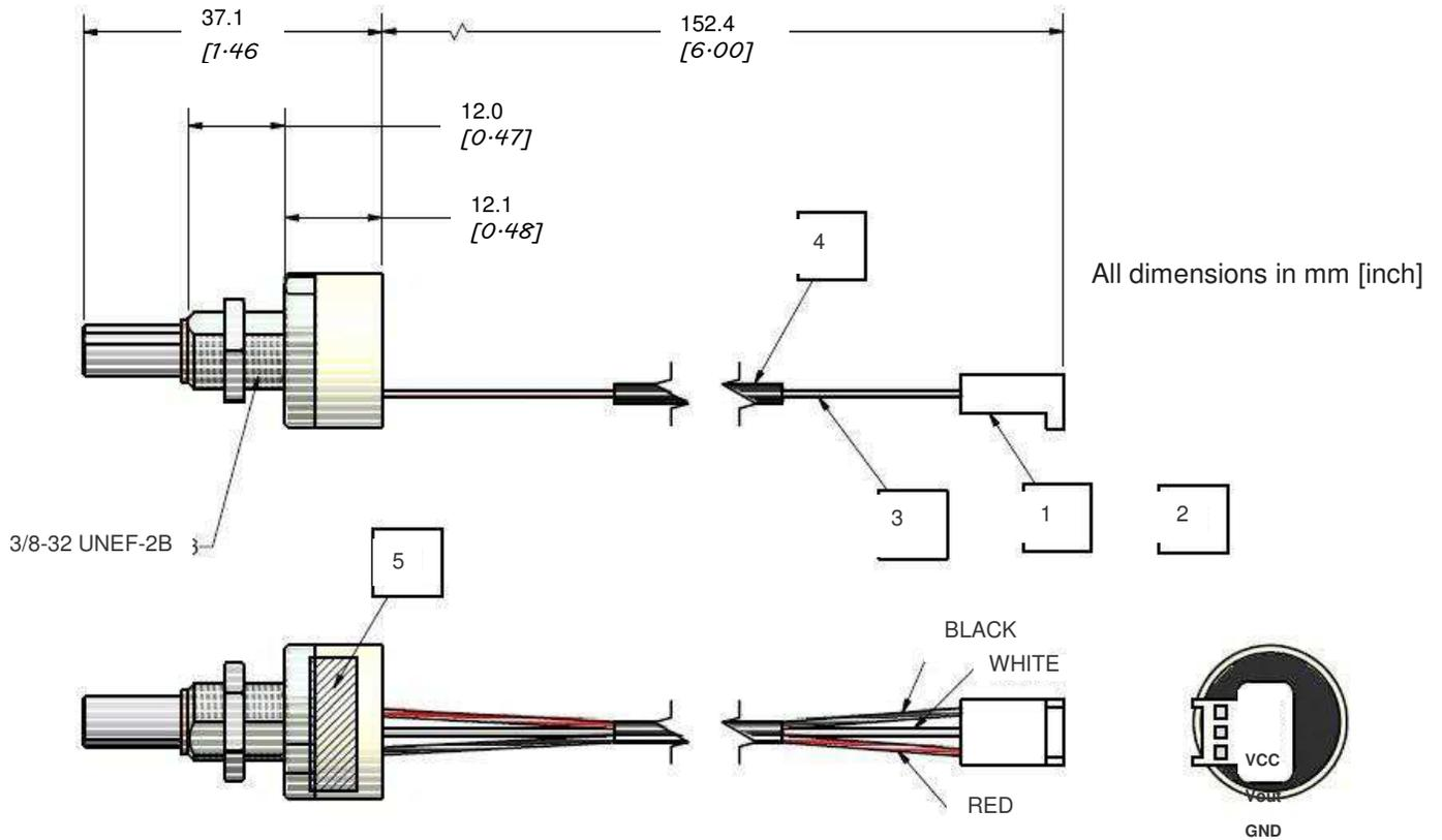
Figure 1: Dimension of the ED-22 (side view)
