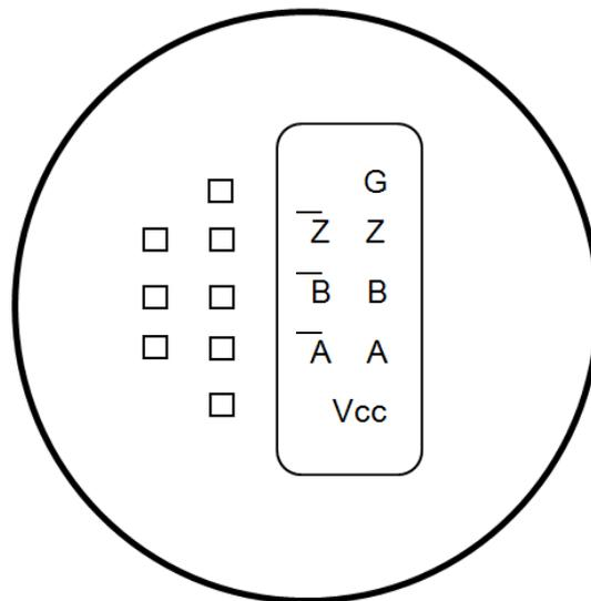
Figure 3: Pinning of the ED-20 (HVD and LVD)
