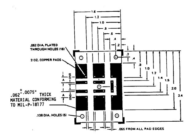
(a) "A" dimension -- .200 or .250 inch between hole centerlines, as applicable for connectors being tested.
