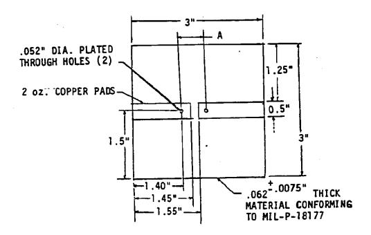
NOTE: (a) "A" dimension -- .200 or .250 inch between hole centerlines, as applicable for connectors being tested.
