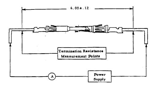
Note: Termination resistance equals millivolts divided by test current less resistance of 4.5 inches of wire.
