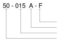
Coating (F = Gel Fill, Blank = No Coating) Type (A = Absolute) Pressure Range Model
