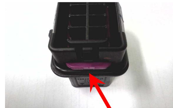
**DETAIL “B”** Locked position of Sec lock.
