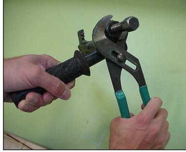
Step 5) Use pliers or similar tool to tighten the screw, completing the assembly.
