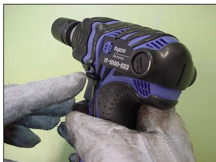
Step 4A) Check electrical tool's rotation direction, before starting the application and, if necessary, change it.
