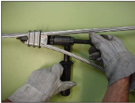
Step 1) Unscrew actuator modules' screw to insert the connector in the application tool.
