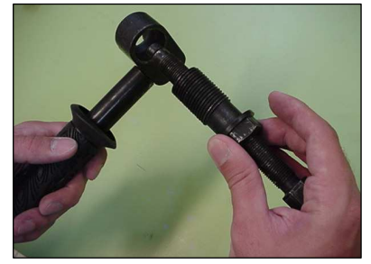
Step 3) Add the actuator module plus washer to the cradle.
