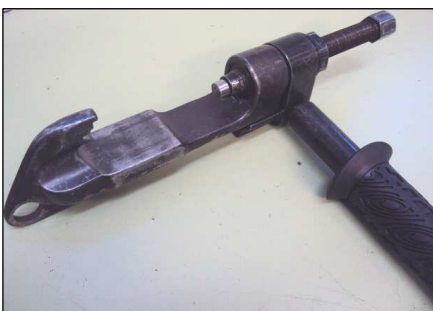
Step 1) Unscrew the actuator modules' screw to the farthest possible.
