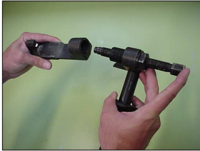
Step 4) Put the actuator module in position and screws it to the head.
