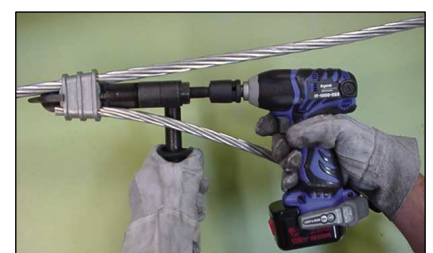
Step 6A) Press the electrical tool's trigger to start the application. On average, the total application's time is 20 seconds.
