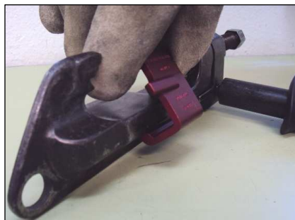
Step 2) Hook the auxiliary red platform over side application tool's head.
