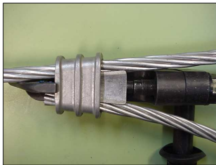
Step 2) Turn back actuator modules' screw until it presses the Wedge component.
