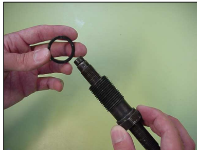
Step 2) Join the washer to actuator module.
