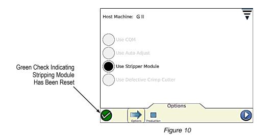
11. Check for proper functioning of the terminator by operating the stripping module in the Step mode. Refer to Paragraph 4.1.
