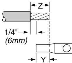
$$\text{"Z" Insulation Cutback} = \text{"Y" Length of Lug Barrel} + \frac{1}{4} \text{" (6mm)}$$
