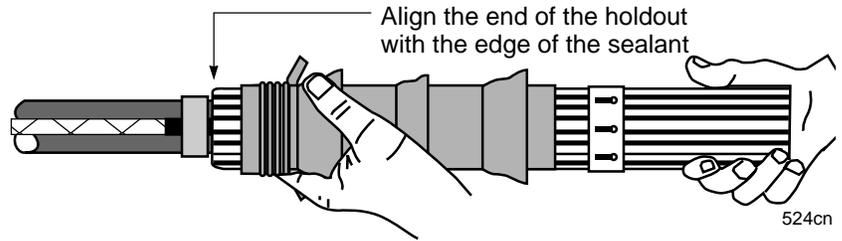
Slide the termination completely off the holdout using a twisting and pulling motion as shown.
