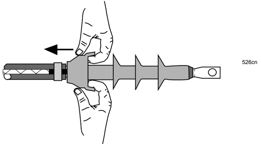
If after installation the termination is not correctly positioned, it is possible to gently slide it into place, so that the final assembly is positioned as shown in the drawing in step 11.
