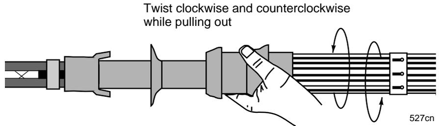
Using the pull tabs, pull the flip-back portion away from the main termination, at the same time working the first two fingers of each hand between the flip back and main termination. Pull the stretched out flip back over the cable jacket and sealant.
