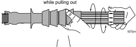
Using the pull tabs, pull the flip-back portion away from the main termination, at the same time working the first two fingers of each hand between the flip-back and main termination. Pull the stretched out flip-back over the cable jacket and sealant.
