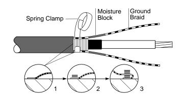
(3) Fold the braids back over the spring clamp wraps. Continue to wrap the remaining clamp over the braids. Tighten clamp by twisting it in the direction it is wrapped and secure with the copper foil tape provided.
