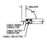
2.0 <u>SHAPE INNER CONDUCTOR OF CABLE</u>
