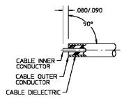
2.0 <u>SHAPE INNER CONDUCTOR OF CABLE</u> 2.1 FILE BLUNT END OF INNER CONDUCTOR TD AN 85°-90° CONE/
