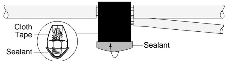
Wrap another layer of black cloth tape over the sealant and around the split bolt as shown.
