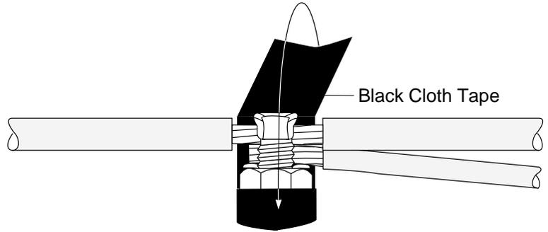
Tear off a 1" (25mm) piece of sealant from the long strip and apply to the split bolt as shown.
