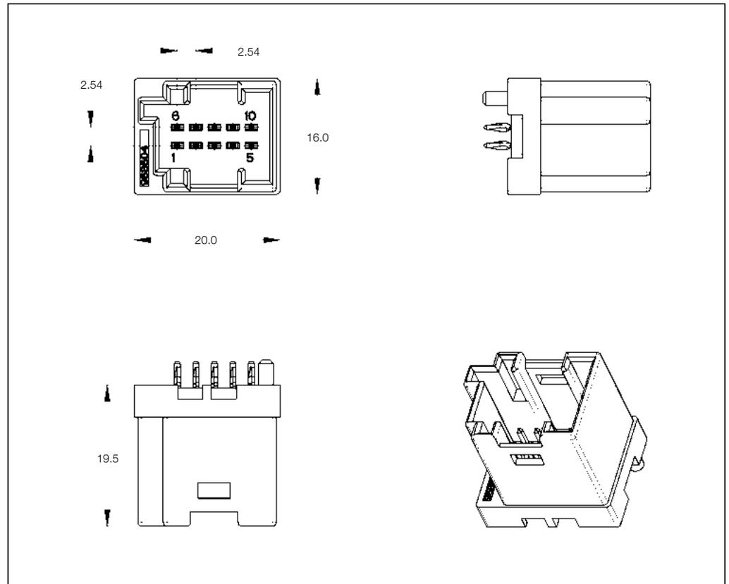
**10 Position PCB Header with ACTION PIN**
