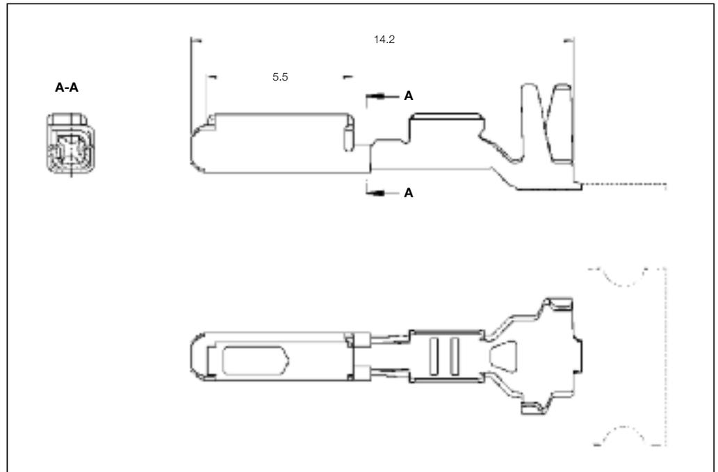
**MQS Clean Body Receptacle Contacts with Single Wire Sealing System**
