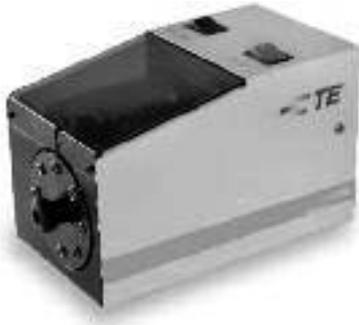
The AT-ST machine strips and twists wires with sizes from 0.03 mm<sup>2</sup> up to 6 mm<sup>2</sup> / AWG 32-10. The adjustable turret head with 8 guide tubes for different wire sizes centralizes positioning of wires. Special ground blades cut and strip special insulations.
