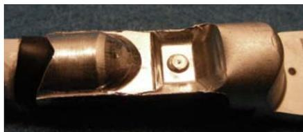
*Under Inserted Terminal (Top View)*
