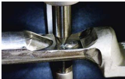
Insulation Barrel Crimp Height Measurement
