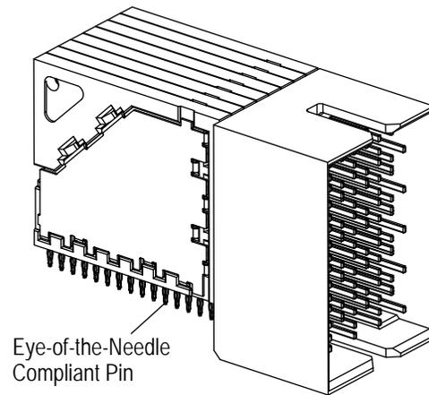
*Right-Angle Press-Fit Pin Header, Left-End Wall
