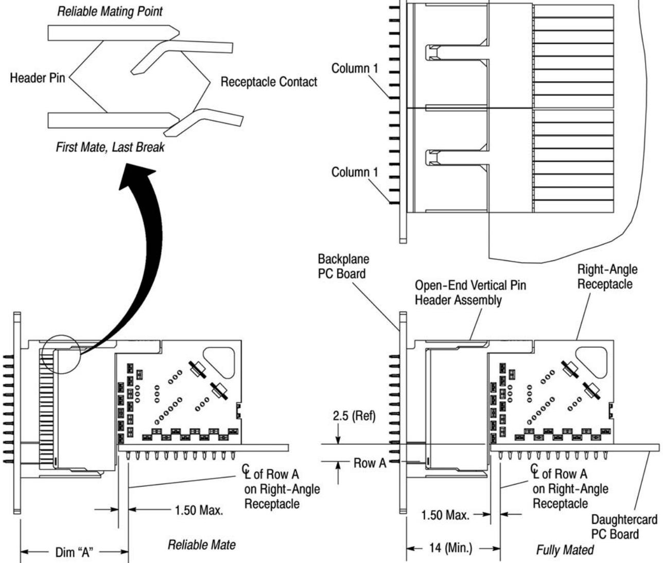
**NOTE:** The first mate, last break sequencing point is the first and last instance in a mating cycle where the pin comes in contact with the beam, but has not deflected the beam. The reliable mating point is the first and last instance in a mating cycle where the pin has completely deflected the beam, and the beam is supplying full normal force to the pin.
