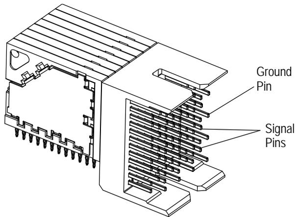
*Right-Angle Press-Fit Pin Header, Open-End
