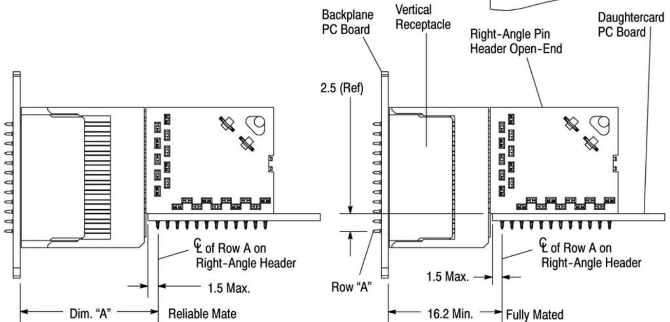
**NOTE:** The first mate, last break sequencing point is the first and last instance in a mating cycle where the pin comes in contact with the beam, but has not deflected the beam. The reliable mating point is the first and last instance in a mating cycle where the pin has completely deflected the beam, and the beam is supplying full normal force to the pin.
