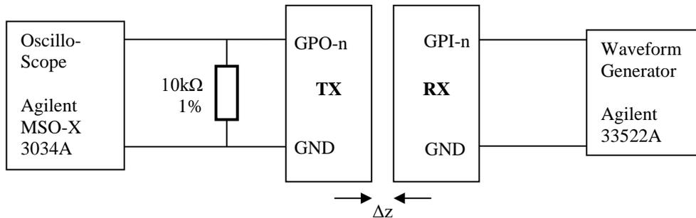
Figure 3.18.1 – Setup for Digital Link Stability Test
