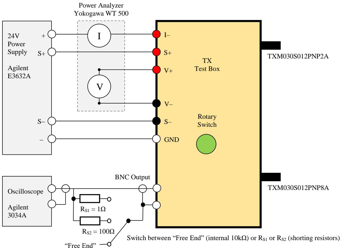
Figure 3.9.4 – Data Link Output Short Circuit Protection and Output Impedance Setup
