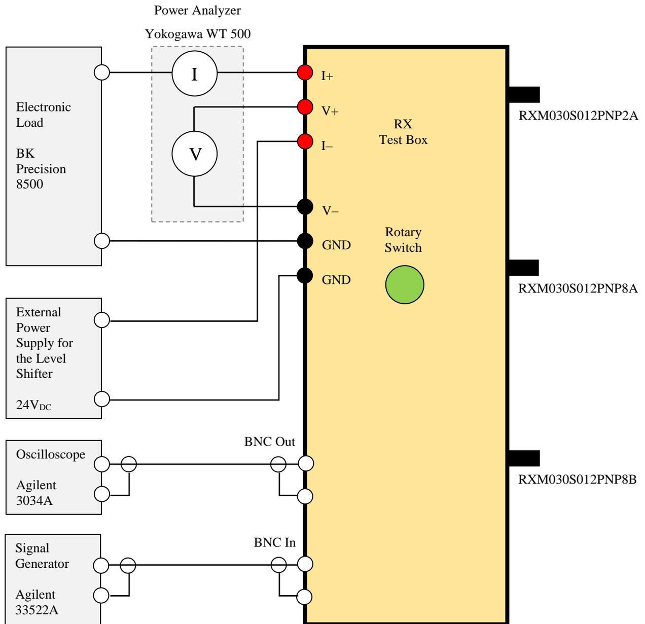
Figure 3.9.5 – RX Test Box Setup
