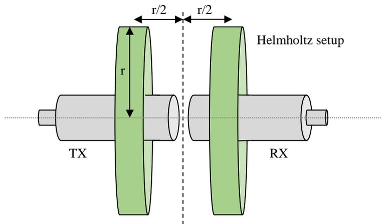
Figure 3.14.1 – External Magnetic Field Measurements Setup
