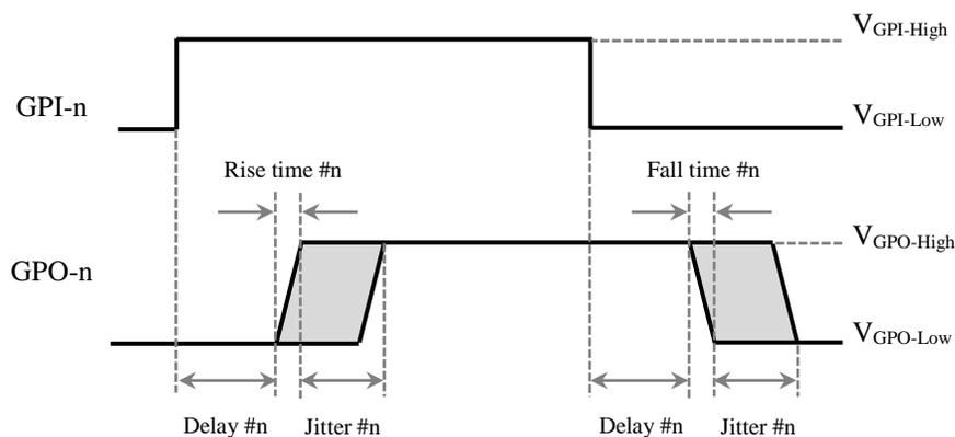
Figure 3.18.2 – Definition of Delay and Jitter for GPIO Link
