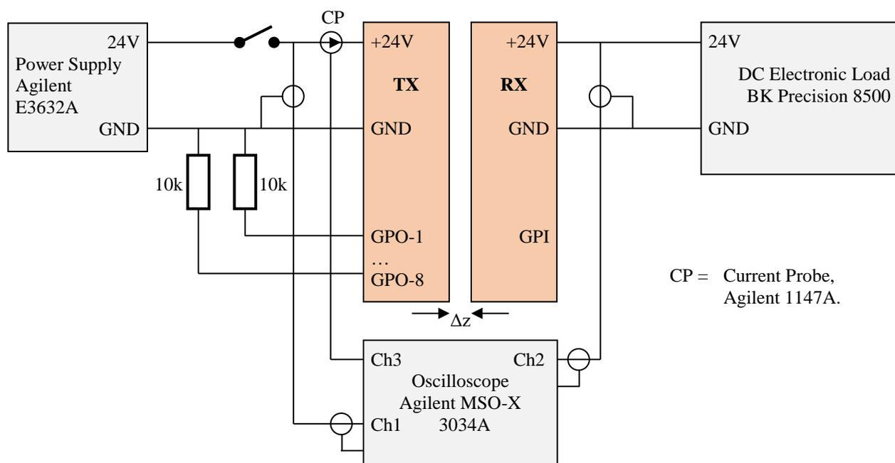
Figure 3.10.1 – Power Link Operational Readiness and Inrush Current Setup
