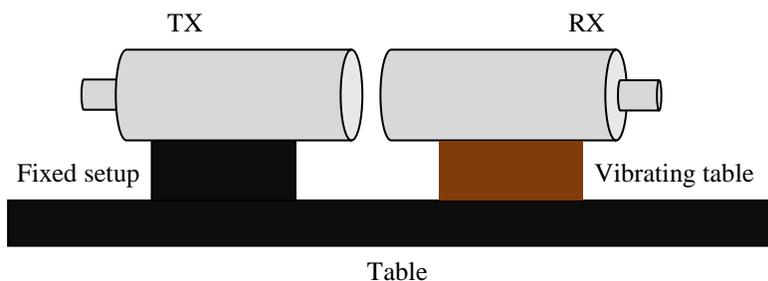
Figure 3.16.1 – Power Link Vibration Performance Measurements Setup
