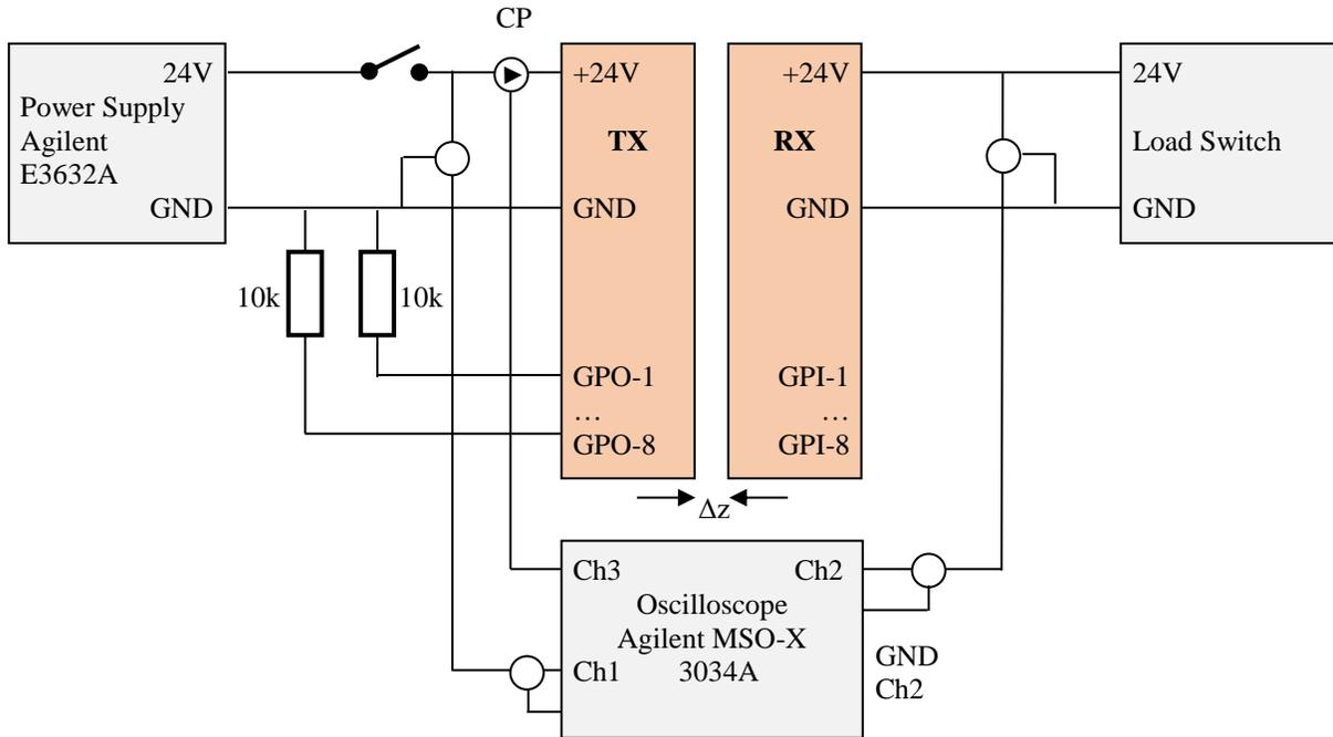
Figure 3.12.1 – Output Inrush Current Setup
