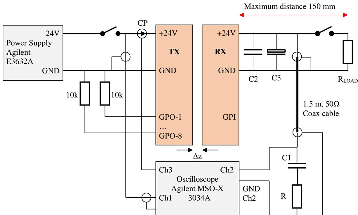
Figure 3.11.1 – Power Link Ripple and Noise Setup
