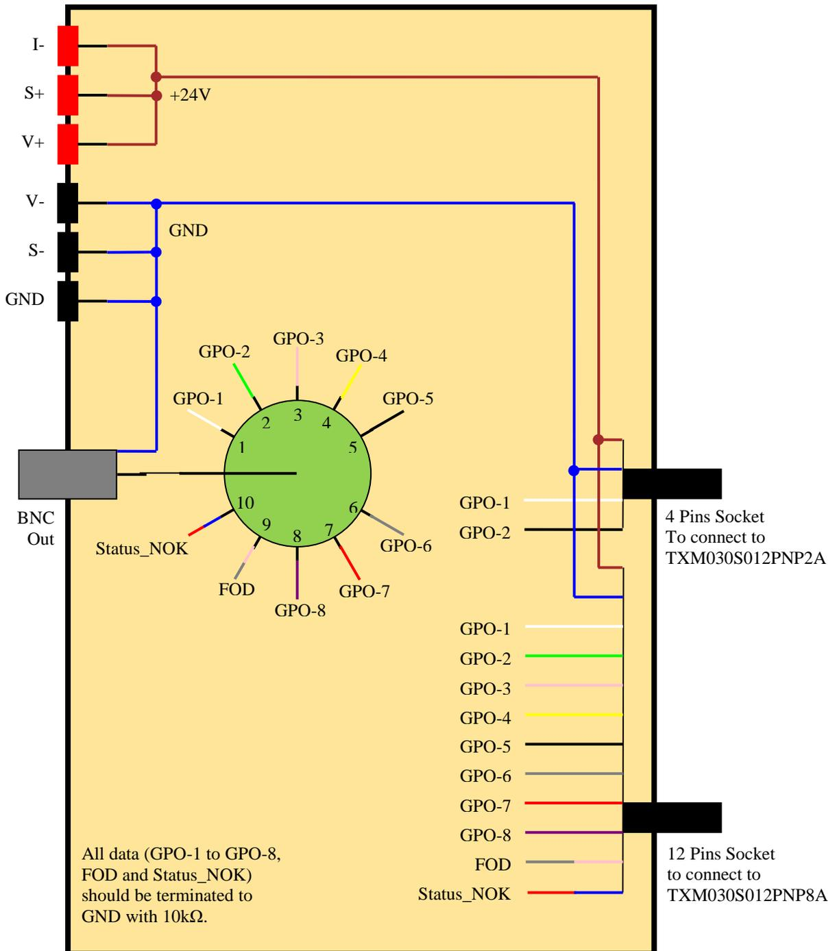
Figure 3.9.1 – TX Test Box
