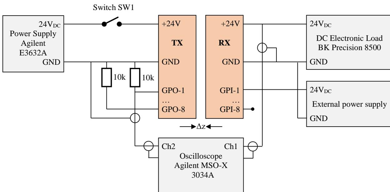
Figure 3.15.1 – Setup for Data Link Operational Readiness
