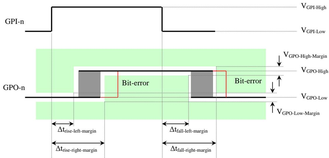
Figure 3.18.3 – Definition of Margins for Bit Error Rate (BER) – GPIO Link Measurements
