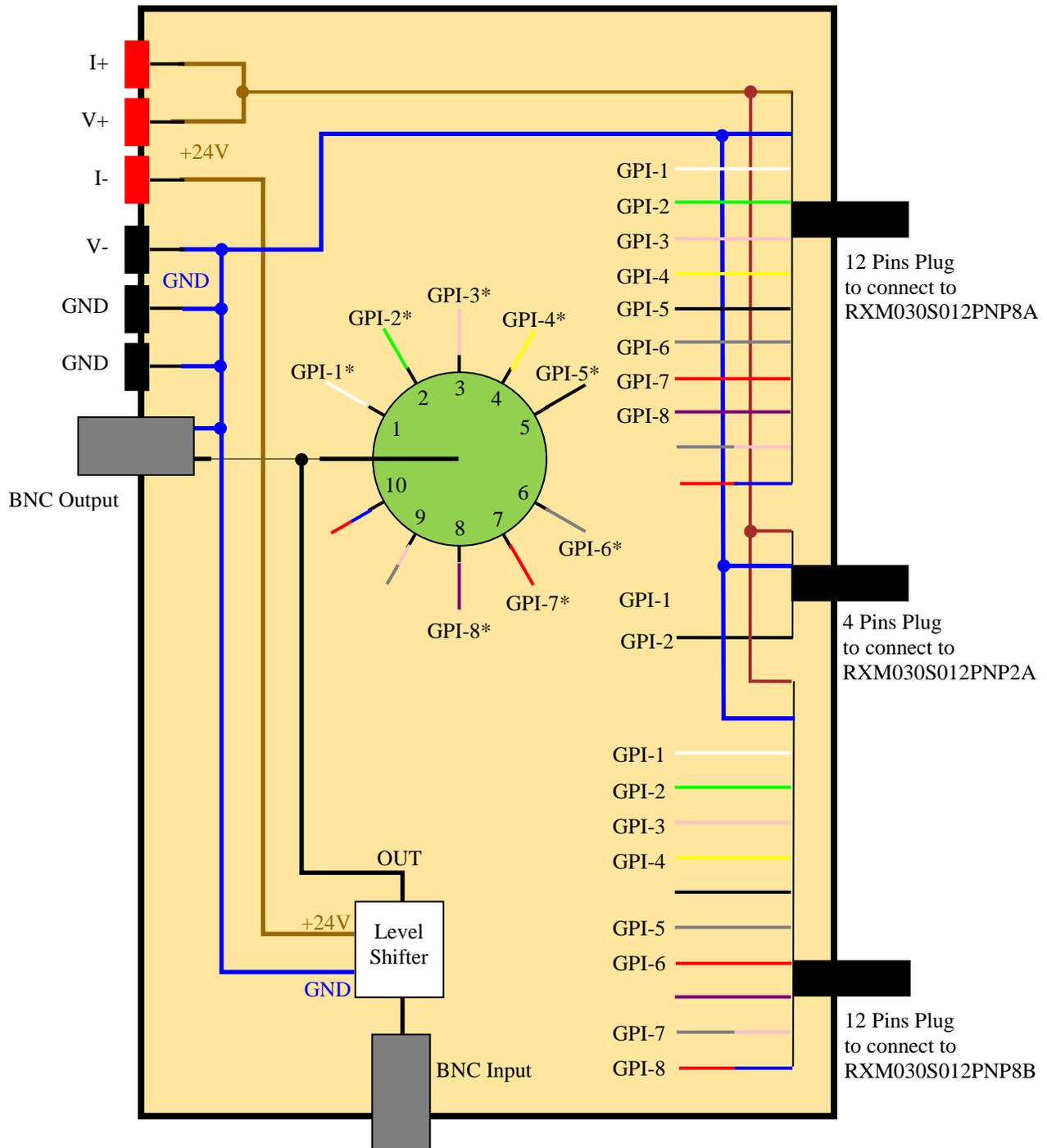
Figure 3.9.2 – RX Test Box
