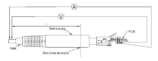
Note: Resistance due to L millimeter of wire shall be removed from all readings.
