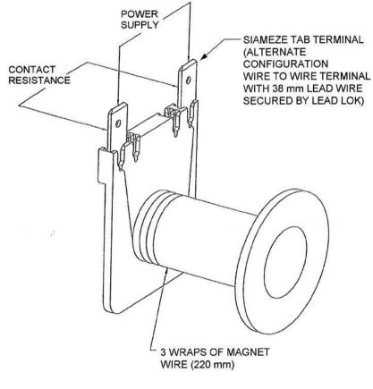
Figure 3 Test Configuration
