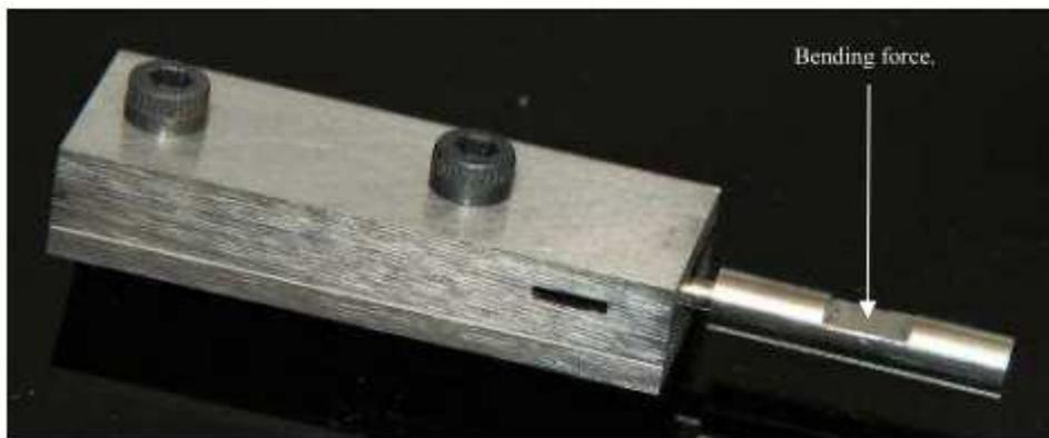
Overview of the adapter used with the rigid steel gauge plug inserted into the connector.
