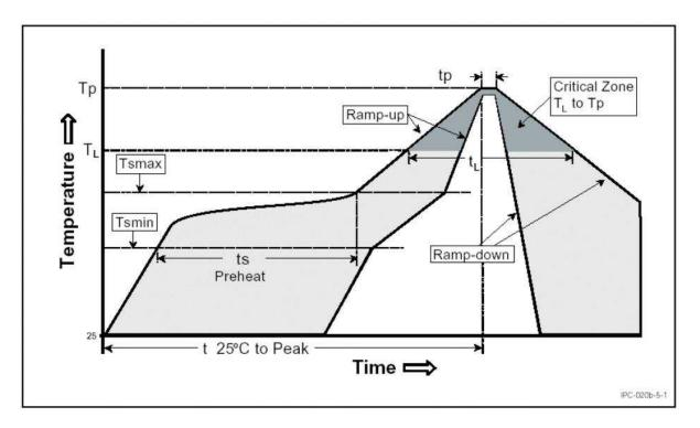
Figure 9. Forced hot air convection (reflow) heat curve.
