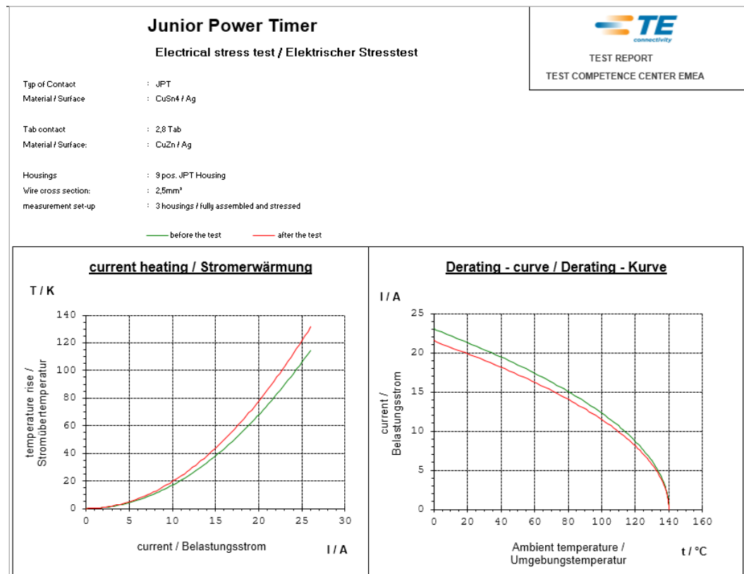
Derating – curve / Derating – Kurve 14
