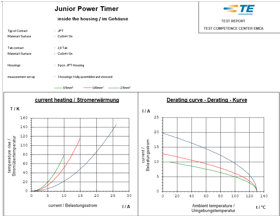
Derating – curve / Derating – Kurve 7
