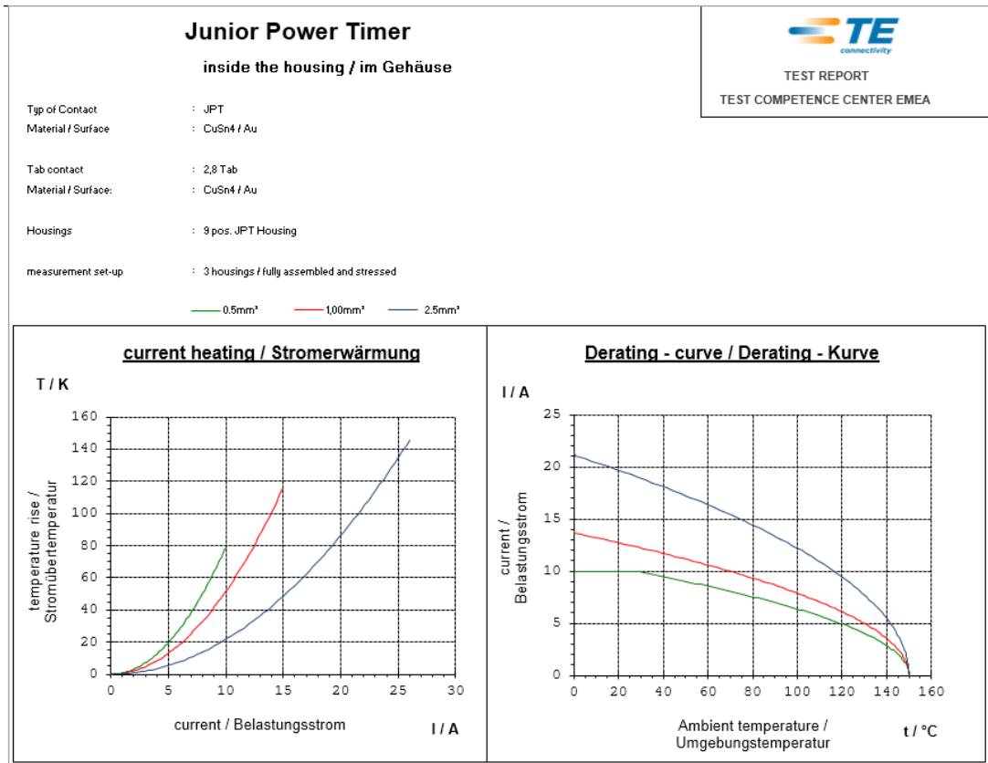
Derating – curve / Derating – Kurve 9
