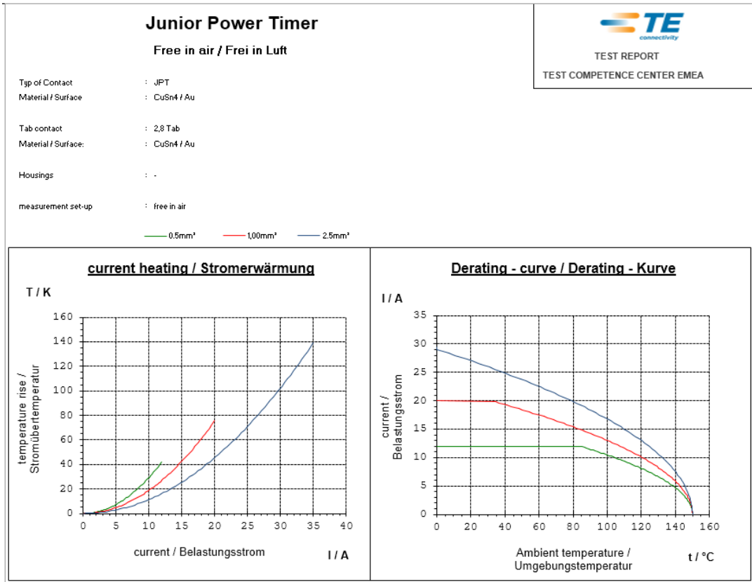
Derating – curve / Derating – Kurve 3
