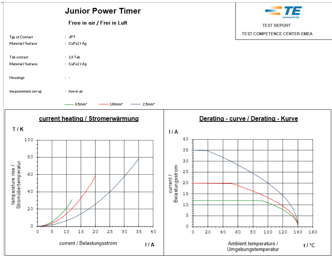
Derating – curve / Derating – Kurve 5
