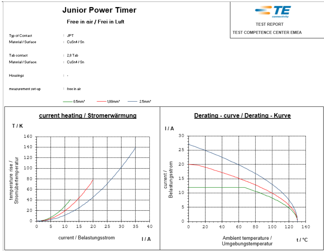
Derating – curve / Derating – Kurve 1
