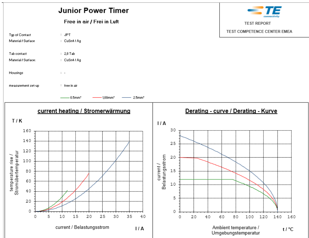
Derating – curve / Derating – Kurve 2
