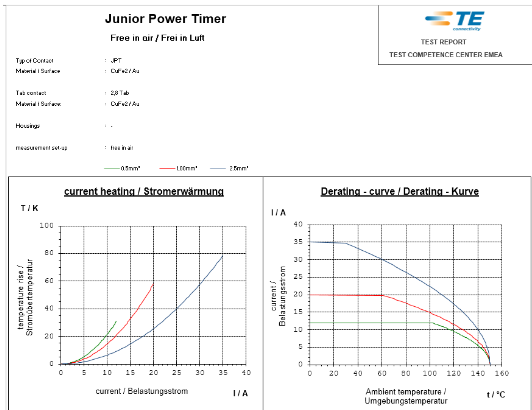
Derating – curve / Derating – Kurve 6
