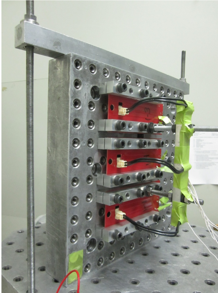
Figure 2 Vibration and Mechanical Shock Mounting Fixture
