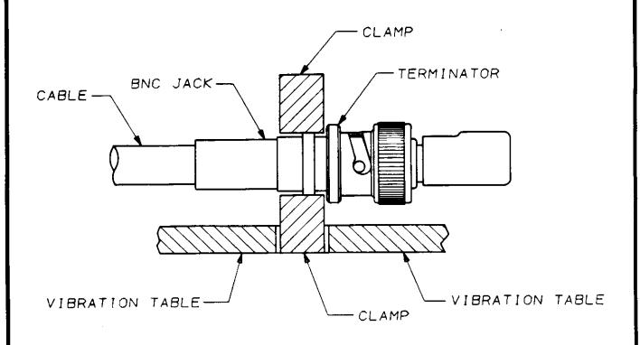
Figure 4 Vibration and Shock
